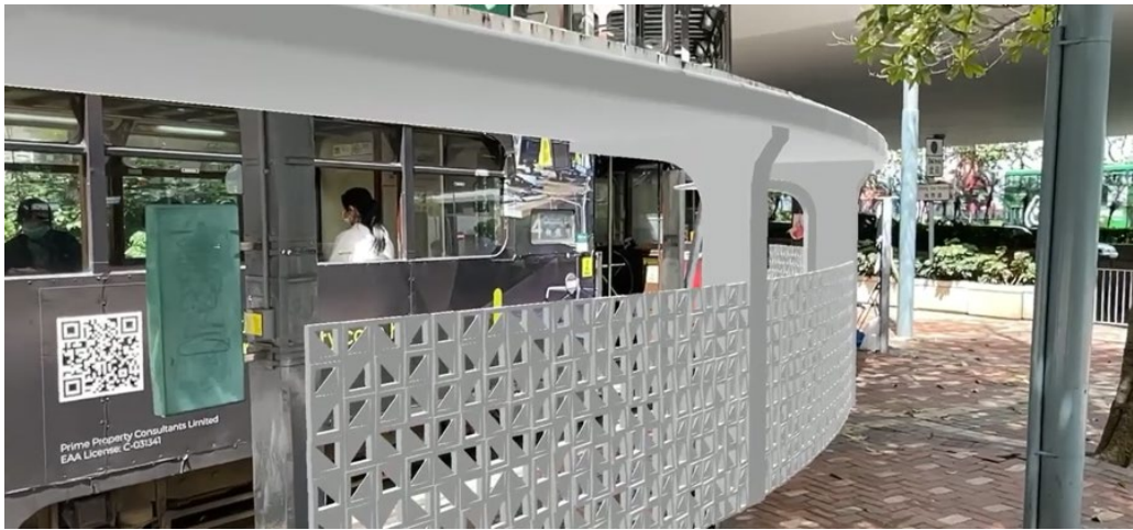
Figure 6. Screenshot of on-site virtual projection of facade patterns through Fologram on Apple iPad
